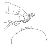
Check the rubber seal in the valve. Turn the valve clock-wise until the valve is firmly connected to the canister. Check for any leaks before igniting stove. Turn the butane canister counter-clockwise to disconnect the stove.
